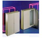
seal, screw-fastened tubular frame with holes on a 25 mm DIN pitch pattern, locking rod with double-bit insert to DIN 43668. (Door hinge may be swapped from right to left in all single-door enclosures). Hinges with captive hinge pins, door opening angle 130° to VDI can be retrofitted to 180°.
