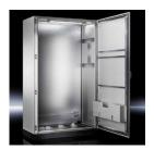
of one-piece construction including side panels and roof. Enclosure section with system punchings on a 25 mm DIN pitch pattern. Vertical sections as well as front and rear roof frame section with two mounting levels for space-saving system installation. Screw-fastened rear panel, welded base assembly consisting of base frame and multi-divided, sliding gland plates, r/h door hinge
