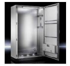
of one-piece construction including side panels and roof. Enclosure section with system punchings on a 25 mm DIN pitch pattern. Vertical sections as well as front and rear roof frame section with two mounting levels for space-saving system installation. Screw-fastened rear panel, welded base assembly consisting of base frame and multi-divided, sliding gland plates, r/h door hinge.
