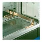
**Technical specifications** Tested short-circuit resistance - PE/PEN combination 30 x 5 mm is: Icw 18 kA, 1 sec - PE/PEN combination 30 x 10 mm is: Icw 30 kA, 1 sec - PE/PEN combination 40/80 x 10 mm: Icw 30 kA, 1 sec; Icw 42 kA, 1 sec (when mounted on blank section frames) For enclosure width: 400 mm Length: 392 mm
