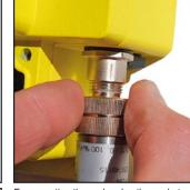
For mounting the probe plug the socket and screw on the sensor by turning the lower knurled thumb clock wise. Just screw hand tight. A small clearance between ExCos-D (transducer) and ExPro-C... (probe) has to be accepted due to production conditions.
