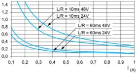
DC13switching electromagnets, L/R ≤ 2 x (Ue x le) in ms, Ue: rated operational voltage, le: rated operational current (with a protective diode on the load, DC12 curves must be used with a coefficient of 0.9 applied to the number in millions of operating cycles)
