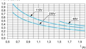
AC15control of electromagnetic loads > 72 VA, make:  $\cos \phi$  = 0.7, break:  $\cos \phi$  = 0.4.
