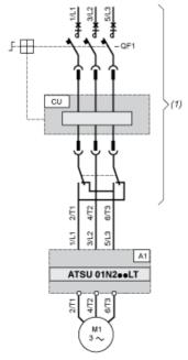
(1) TeSys U with reversing unitA1: Soft start/soft stop unitQF1:TeSys U controller-starterCU: TeSys U control unit
