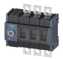
Switch disconnector 80 A, Size 2, 3-pole Front operating mechanism left Basic unit without handle flat terminal incl. phase barriers
