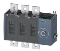
Switch disconnector 630 A, Size 4, 3-pole Side operating mechanism right Basic unit without handle flat terminal
