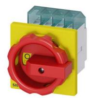
SENTRON, Switch disconnector 3LD, emergency switching-off switch, 4-pole, Iu: 16 A, operating power / at AC-23 A 400 V: 7.5 kW, front-mounted, rotary operating mechanism, Red / yellow, 4-hole mounting of the handle
