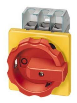
EMERG. STOP SWITCH 3-POLE IU=16, P/AC-23A AT 400V=7.5KW FRONT MOUNTING CENTER HOLE MOUNTING ROTARY ACTUATOR RED/YELLOW (EMERG. STOP)
