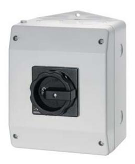
3-P. MAIN CTR. SWITCH IU=16, P/AC-23A AT 400V=7.5KW 1 N-TERMINAL + 1 PE-TERMINAL MOULDED-PLASTIC ENCLOSED, IP65 ROTARY ACTUATOR BLACK
