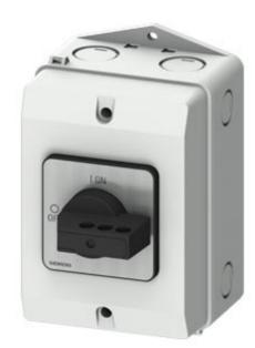
SENTRON switch disconnector 3LD in molded-plastic enclosure, repair and maintenance switch with EMC plate, 3-pole lu: 16A, AC23A 400V at 50/60Hz: 7,5kW, used with frequency converter: AC20 400V at 0-550Hz: 4kW, 1NO + 1NC 20-150ms leading, molded-plastic encapsulation for metric cable gland, knob-operated mechanism, black, lockable in 0- and I-position, incl. cable shield clamps
