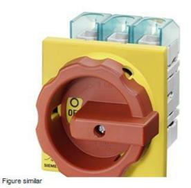
EMERG. STOP SWITCH 3-POLE IU=25, P/AC-23A AT 400V=9.5KW FRONT MOUNTING CENTER HOLE MOUNTING ROTARY ACTUATOR RED/YELLOW (EMERG. STOP)
