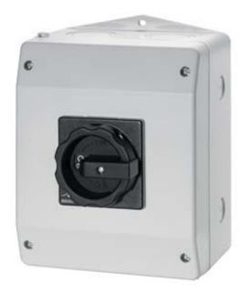
MAIN CONTROL SWITCH 3-POLE IU=25, P/AC-23A AT 400V=9,5KW 1NO+1 NC, 1 N-TERMINAL ENCAPSUL.IN M.P.ENCLOSURE, IP65 ROTARY ACTUATOR BLACK METRIC THREAD
