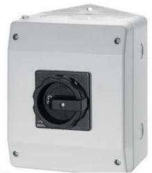
MAIN SWITCH 6-POLE IU=25, P/AC-23A AT 400V=9,5KW 1NO+1NC, 1 N-TERMINAL MOULDED-PLASTIC ENCLOSURED, IP65
