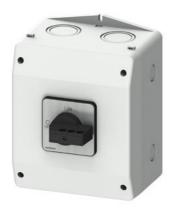
SENTRON switch disconnector 3LD in molded-plastic enclosure , repair and maintenance switch with EMC plate, 6-pole lu: 25A, AC23A 400V at 50/60Hz: 9,5kW, used with frequency converter: AC20 400V at 0-550Hz: 5,5kW, 1NO + 1NC 20-150ms leading, molded-plastic encapsulation for metric cable gland, knob-operated mechanism, black, lockable in 0- and I-position, incl. cable shield clamps
