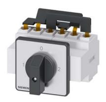
SENTRON, Switch disconnector 3LD, change-over switch, 3-pole, lu: 32 A, Operating power / at AC-23 A at 400 V: 11.5 kW, front-mounted, knob-operated mechanism, black, 4-hole mounting of the handle
