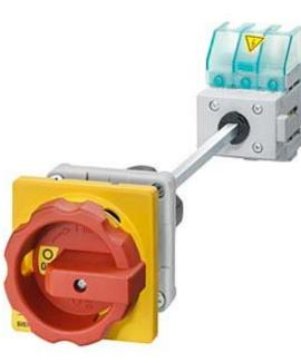
EMERG. STOP SWITCH 3-POLE IU=32, P/AC-23A AT 400V=11.5KW FLOOR MOUNTING DIN RAIL/TWO-HOLE MOUNTING ROTARY ACTUATOR RED/YELLOW (EMERG. STOP)
