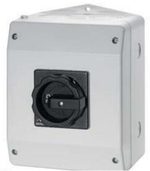
MAIN SWITCH 6-POLE IU=32, P/AC-23A AT 400V=11,5KW 1NO+1NC, 1 N-TERMINAL MOULDED-PLASTIC ENCLOSURED, IP65
