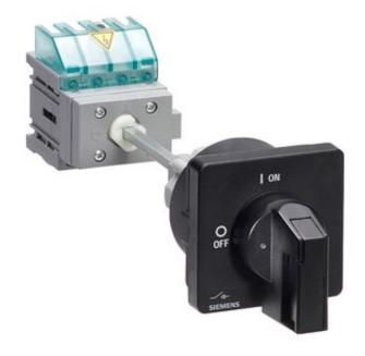
IU=160A, P/AC-23A BEI 400V=75KW SWITCHING ELEM. FLOOR MOUNTING WITH DOOR-COUPL. ROT. OP. MECH. CONTROL ELEMENT BLACK FRONT / 4-HOLE MOUNTING 6-POLE
