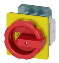
SENTRON, Switch disconnector 3LD, emergency switching-off switch, 3-pole, lu: 63 A, operating power / at AC-23 A 400 V: 22 kW, front-mounted, 1 NC, 1 NO, rotary operating mechanism, Red / yellow, 4-hole mounting of the handle
