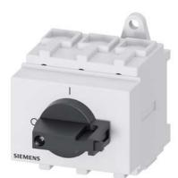
SENTRON, Switch disconnector 3LD, main switch, 3-pole, lu: 63 A, Operating power / at AC-23 A at 400 V: 22 kW, installation in distribution boards, knob-operated mechanism, black, handle direct at the switch
