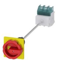
SENTRON, Switch disconnector 3LD, emergency switching-off switch, 3pole, Iu: 63 A, operating power / at AC-23 A 400 V: 22 kW, floor mounting with door coupling, rotary operating mechanism, Red / yellow, central mounting 22.5 mm of the handle
