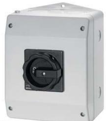
MAIN SWITCH 6-POLE IU=63, P/AC-23A AT 400V=22KW 1NO+1NC, 1 N-TERMINAL MOULDED-PLASTIC ENCLOSURED, IP65
