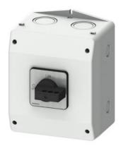
SENTRON switch disconnector 3LD in molded-plastic enclosure, repair and maintenance switch with EMC plate, 3-pole lu: 63A, AC23A 400V at 50/60Hz: 22kW, used with frequency converter: AC20 400V at 0-550Hz: 18,5kW, 1NO + 1NC 20-150ms leading, molded-plastic encapsulation for metric cable gland, knob-operated mechanism, black, lockable in 0- and I-position, incl. cable shield clamps and hose clamps
