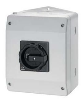
MAIN CONTROL SWITCH 3-POLE IU=125, P/AC-23A AT 400V=45KW 1 N-TERMINAL + 1 PE-TERMINAL ENCAPSUL.IN M.P.ENCLOSURE, IP65 ROTARY ACTUATOR BLACK METRIC THREAD
