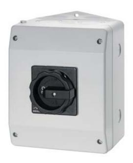
MAIN CONTROL SWITCH 3-POLE IU=125, P/AC-23A AT 400V=45KW 1NO+1 NC, 1 N-TERMINAL ENCAPSUL.IN M.P.ENCLOSURE, IP65 ROTARY ACTUATOR BLACK METRIC THREAD
