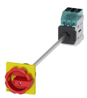
Load disconnector 3LD3, Iu 40 A Main switch 3-pole Rated operating capacity at AC-23 A at 400 V 15.0 kW floor mounting Basic switch with door coupling Central hole mounting 22.5mm Rotary actuator red / yellow 66 x 66 mm
