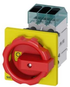
Load disconnector 3LD3, Iu 40 A Main switch 3-pole Rated operating capacity at AC-23 A at 400 V 15.0 kW Front plate mounting Basic switch with Central hole mounting 22.5mm Toggle drive red / yellow 66x66 mm
