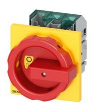
SENTRON, Molded case switch 3LD5 UL, Emergency switching-off, 3-pole, certified according to UL489 UL60947-4-1 and IEC60947-3, UL: 30A, SCCR 50kA at 480VAC, Operating power at 480VAC 3-phase: 20hp, IEC: 32A, Operating power at AC-23A at 400V: 15kW, front-mounted, rotary operating mechanism, red/yellow, 4-hole mounting of the handle, incl. terminal covers for the infeed side
