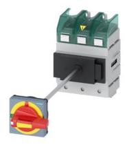
SENTRON, Molded case switch 3LD5 UL, Emergency switching-off, 3-pole, certified according to UL489 UL60947-4-1 and IEC60947-3, UL: 100A, SCCR 65kA at 480VAC, Operating power at 480VAC 3-phase: 60hp, IEC: 100A, Operating power at AC-23A at 400V: 45kW, floor mounting with door coupling rotary operating mechanism, defeatable, emergency switching-off, 4-hole mounting of the handle, without tolerance compensation, incl. terminal covers for the infeed side
