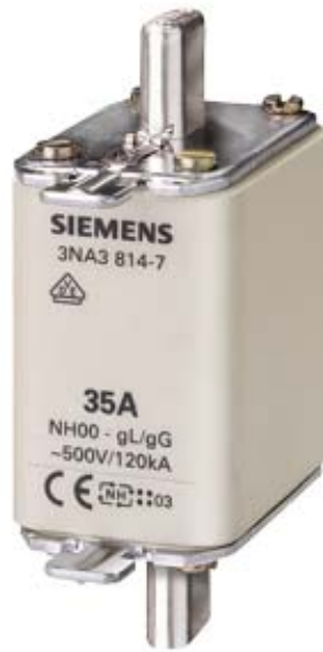
LV HRC FUSE LINK GL/GG WITH NON-INSULATED GRIP LUGS WITH FRONT INDICATOR SIZE 00, 35A, AC 500V/DC 250V
