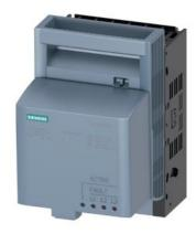
SENTRON, Fuse switch disconnector 3NP1, 3-pole, NH000, 160 A, for assembly and installation on Mounting plate, box terminal, Fuse monitoring: electronic EFM10, Cover level 45 mm  $\,$
