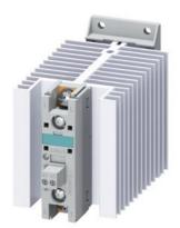
Solid-state contactor 1-phase 3RF2 AC 51 / 50 A / 40  $^{\circ}\text{C}$  48-600 V / 24 V DC Ring cable connection
