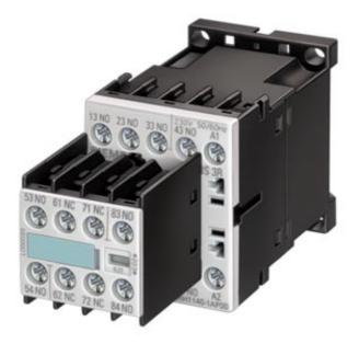
CONTACTOR RELAY, 3NO+1NC, AC 230 V, 50 HZ, SCREW CONNECTION, SIZE S00
