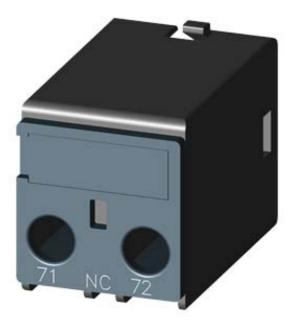
AUX.SWITCH BLOCK,FRONT,1NC, CURR.PATH: 1NC, CONN. F. BELOW, F. CONT. RELAYS A. MOTOR CONT., SZ S00 AND S0, SCREW TERMINAL 71 / 72
