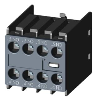
AUX.SWITCH BLOCK,FRONT,4NO, CURR.PATH: 1NO, 1NO, 1NO, 1NO, F. CONT. RELAYS A. MOTOR CONT., SZ S00 AND S0, SCREW TERMINAL .3 / .4,.3 / .4,.3 / .4,.3 / .4
