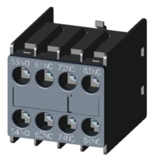
AUX. SWITCH BLOCK , 3NO+1NC COND. PATHS: 1NO, 1NC, 1NO, 1NO, FOR CONTACTOR RELAYS SZ S00, SCREW TERMINAL DIN EN 50011
