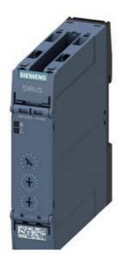
TIME RELAY, MULTI-FUNCTION, 2 CO CONT., 13 FUNCTIONS, 7 TIME SET. RANGES,(1,10,100)S; 10MIN; (1,10,100) HR (S/MIN/HR), 24... 240 V AC/DC, AT AC 50/60HZ, PD AND GOLD- PLATED RELAY CONT., LED, SCREW TERMINAL
