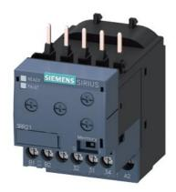
Monitoring relay, can be mounted to Contactor 3RT2, Size S00 basic, analog adjustment Apparent current monitoring 1.6-16 A, 20-400 Hz, 2-phase Supply 24 V AC/DC 1 change-over contact Monitoring for Current overshoot and undershoot Phase failure, Cable break with or without fault buffer ON delay 0-60 s Noise pulse suppression 0-30 s Switching hysteresis 6% Screw connection system
