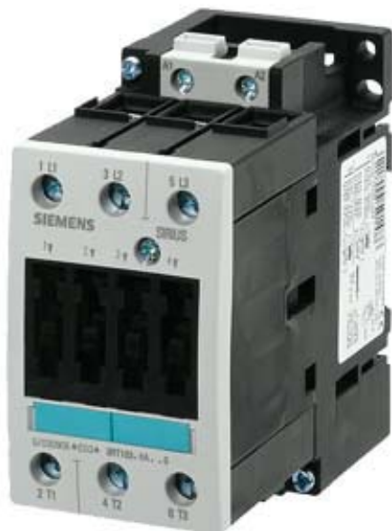
CONTACTOR, AC-3 18,5 KW/400 V, AC 230V 50/60HZ 3-POLE, SIZE S2, SCREW CONNECTION
