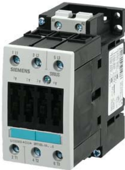
CONTACTOR, AC-3 22 KW/400 V, AC 230 V, 50/60 HZ, 3-POLE, SIZE S2, SCREW CONNECTION
