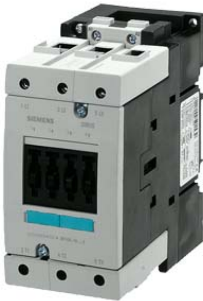
CONTACTOR, AC-3 30 KW/400 V, AC 230V 50/60HZ 3-POLE, SIZE S3, SCREW CONNECTION
