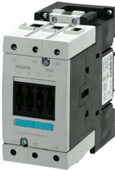
CONTACTOR, AC-3 37 KW/400 V, AC 230V 50/60HZ 3-POLE, SIZE S3, SCREW CONNECTION
