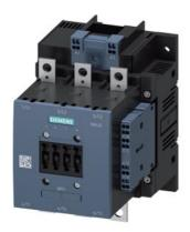
power contactor, AC-3e/AC-3 185 A, 90 kW / 400 V AC (50-60 Hz) / DC Uc: 220-240 V 3-pole, auxiliary contacts 2 NO + 2 NC drive: conventional main circuit: busbar control and auxiliary circuit: spring-loaded terminal
