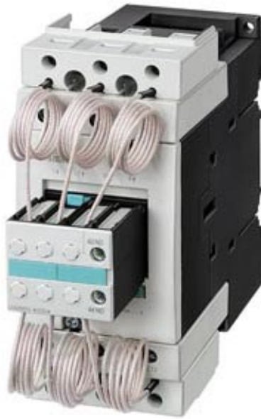
CAPACITOR SW. CONTACTOR, AC-6, 50KVAR/400V, 230V, 50HZ, 3-POLE, SIZE S3
