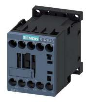
power contactor, AC-3e/AC-3, 9 A, 4 kW / 400 V, 3-pole, 24 V DC, auxiliary contacts: 1 NO, screw terminal, size:  $\rm S00$
