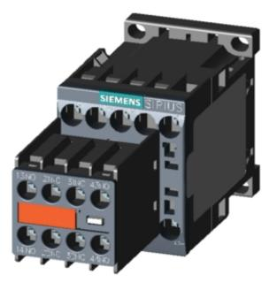
CONTACTOR, AC-3, 4KW/400V, 2NO+2NC, DC 24V, W. INTEGRATED DIODE 3-POLE, SZ S00 SCREW TERMINAL PERMANENT AUX. SWITCH
