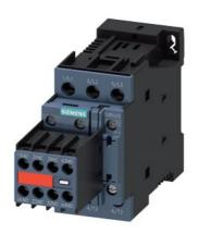
power contactor, AC-3e/AC-3, 9 A, 4 kW / 400 V, 3-pole, 24 V DC, with plugged-in diode combination, auxiliary contacts: 2 NO + 2 NC, screw terminal, captive auxiliary switch
